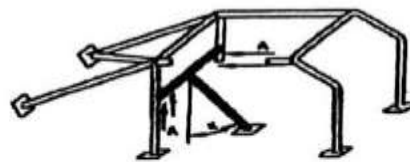
Ⓑ Angle minimum 30° Minimum angle 30°
